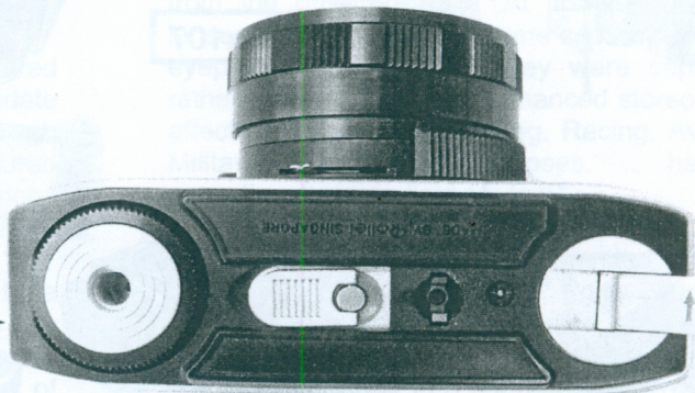
Base with tripod bush left. Back-base lock centre. Fold-out rewind right.
