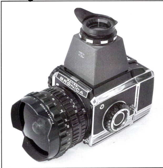
Above..When mounted it is quite compact. Actually no larger than the 40mm or 105mm Bronica-Nikkors. Above right..Note that it focuses to a close 1.5 feet. Below..The built-in gelatin filter holder exposed. Such a system would be necessary on a lens with a large curved front element.
