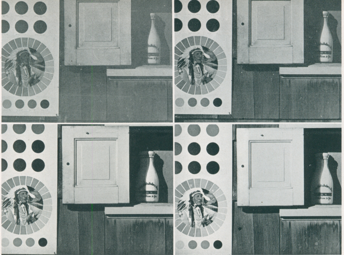
Illustration No. 3. DuPont Parpan developed in Eastman Ultra Fine. Upper left: exposed at Weston 64, flat. Upper right: exposed at Weston 32, good. Lower left: exposed at Weston 16, very good. Lower right: at Weston 8, hard.
