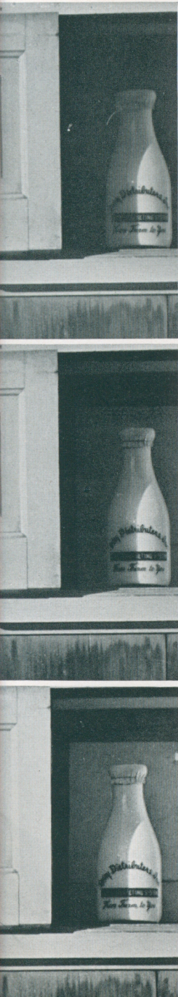
Right: Illustration No. 5. 55X enlargements of all films developed in Edwal 20. Left, top to bottom: DuPont Superior, Eastman Super X, Eastman S. S. Pan, and Agfa Superpan. Right, top to bottom: Eastman Panatomic, DuPont Parpan, Agfa Finopan, DuPont Micropan, and Agfa Plenachrome.
