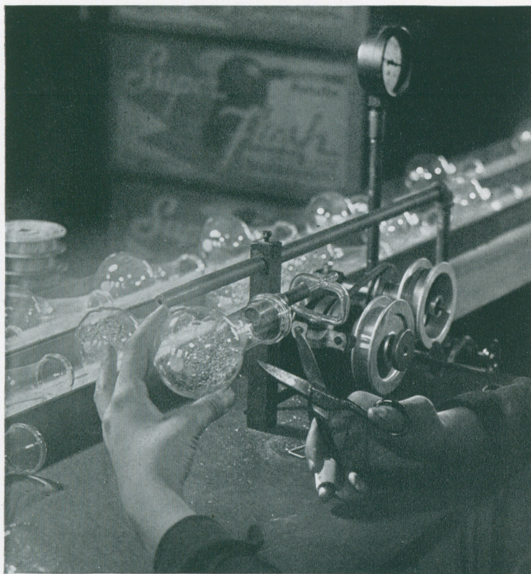
Facing page: Lacquering machine spraying a coating of lacquer on inside of bulb. Above: Automatic crimping and measuring machine which measures and blows spun hydronalium wire into the bulb. Right: Mounting machine which clamps the tungsten-wire filament between the two nickel terminals of the lead-in wires.
