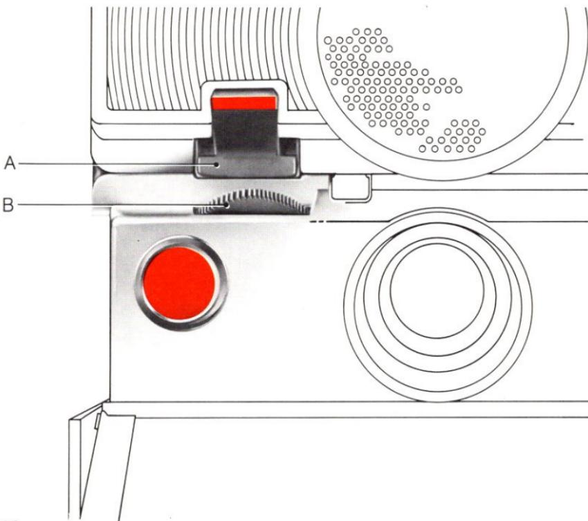
**To use the focus wheel:** Look at the most important part of the scene. Roll the wheel all the way in one direction, then all the way in the other. Notice that the image changes from fuzzy to sharp and back to fuzzy.
