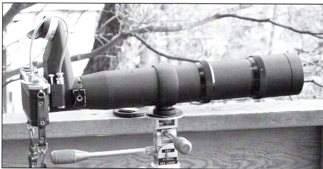
50cm/f8 Fernobjektiv manufactured in 1948 in the PANFLEX mount.
