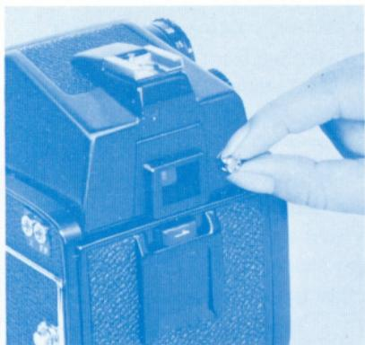
1. Turn the finder release button clockwise until it stops (about 60°), so that the white dot on the button is aligned with the white dot on the finder. Then you will be able to push in on the release button.
