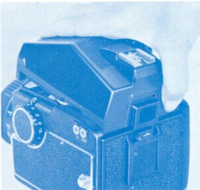
2. While pushing in on the release button with your thumb, lift the finder off the camera body.
