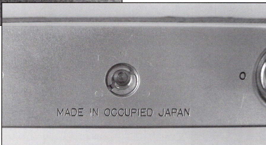
Fig. 10e (below)...The riveted type socket results in a baseplate where the rivets can be seen, albeit faintly.
