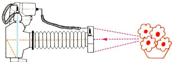
Flash exposure with ringlight and bellows would normally require complex calculations, including bellows factors and the like. But with the Auto 622 and cameras which have dedicated through-the-lens exposure metering, it's all automatic. The camera reads the flash, just as it does "continuous" light.
