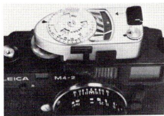
Leica MR-4 meter slides into hot shoe. Pin on meter couples to shutter-speed dial.
