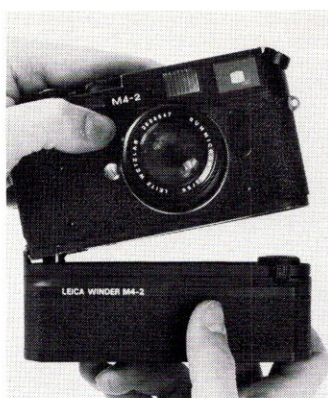
After removing baseplate, M4-2 winder can be attached, but of course you must remove film first, or fog it.
