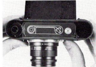
Diagram shows how to load film. Place cartridge at left and leader through slot in take-up spool.
