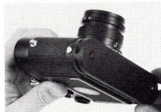
Lift and turn key at right to remove baseplate (rather than opening the back) to load film.
