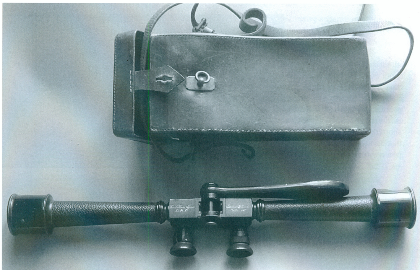
An early Zeiss 10x Relief Fernrohr , which, with detail improvements, became the 10x Teleplast when the roof-prism version was introduced.
