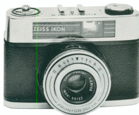
Contina LK (10.0637) 1963-1965 24x36mm exposures on 35mm film; Color-Pantar 45mm f2.8 lens in Prontor 250LK shutter
