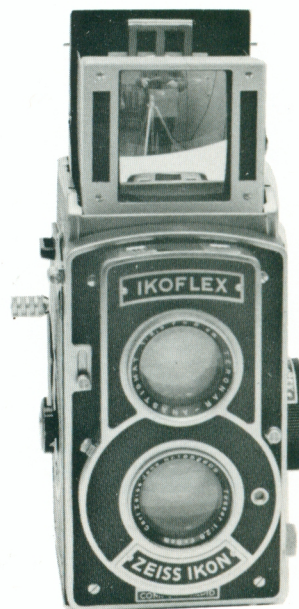
Ikoflex III (853/16) 1939-1940 6x6cm exposures on 120 film; Tessar 8cm f2.8 lens in Compur-Rapid shutter
