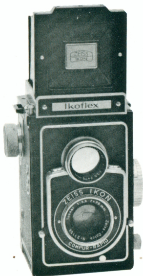
Ikoflex IIa (855/16) 1950-1952 6x6cm exposures on 120 film; Tessar 75mm f3.5 lens in Compur- Rapid shutter
