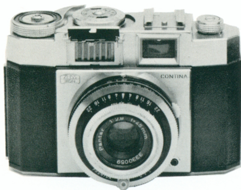
Contina III (529/24) 1955-1958 24x36mm exposures on 35mm film; convertible Pantar 45mm f2.8 lens in Prontor-SVS shutter
