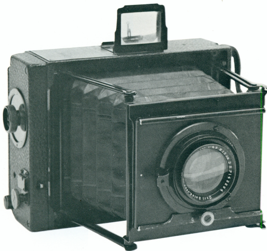
Minimum Palmos Ca. 1905 Carl Zeiss, Jena 9x12cm plates; Tessar 15cm f4.5 lens
