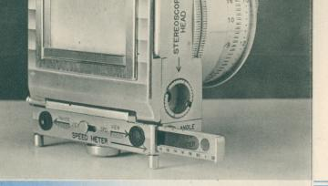
THE COMPASS UNIT SYSTEM ensures correct photography automatically. It is based upon the Extinction Exposure-Meter built into the View-finder of the camera and calibrated in conjunction with the shutter speeds, lens stops and filters. The correct exposure under any lighting conditions and with any combination of stops and filters is arrived at instantly and with no more calculation than is involved in adding 2 and 2 to 4.
