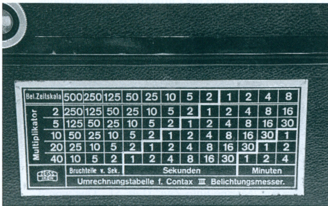
Fig. 3) Details of the back of the unique Contax III (serial number M. 34905) with the conversion plate added to the back of the camera, instead of being nailed onto the back of the leather case. Note that this camera does not show a MF number engraved, neither on the camera or on the lens.
