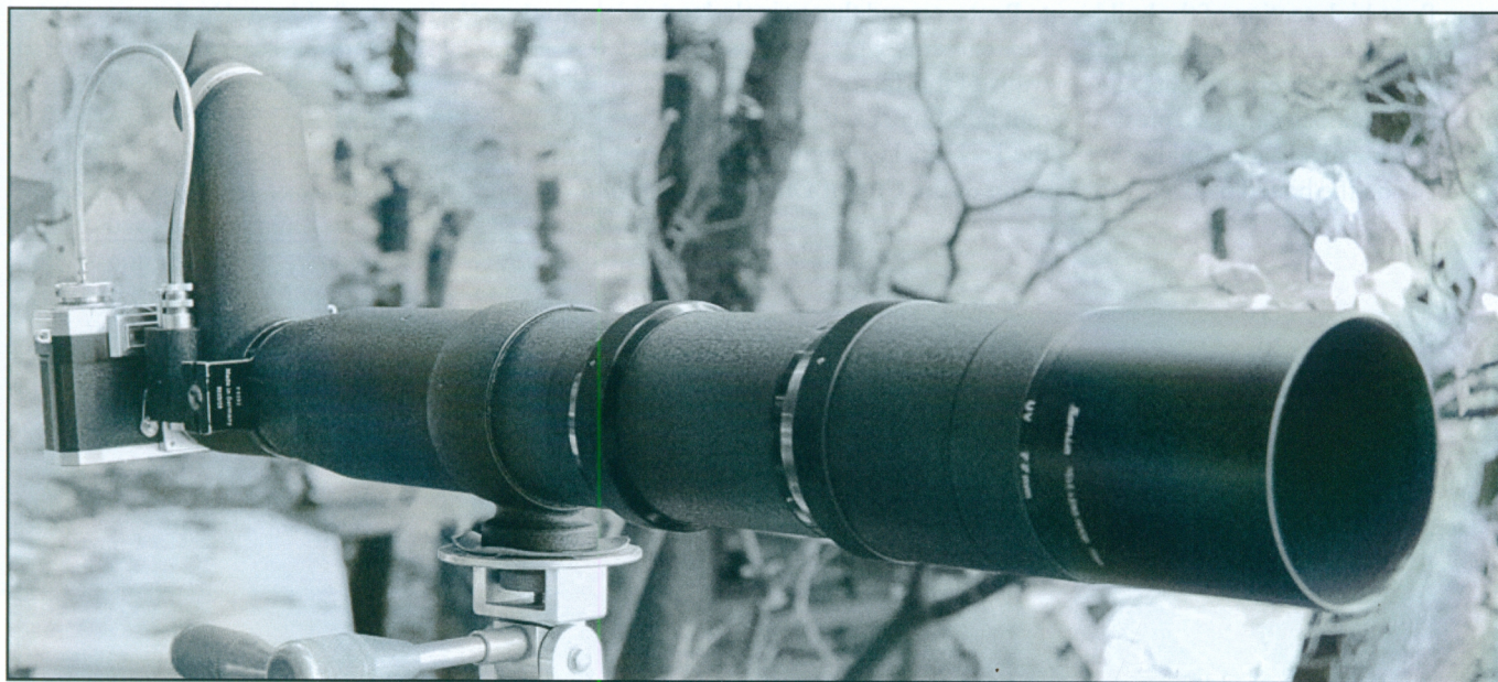
The 500 mm f/8 Fernobjektiv mounted via a Panflex on a Contax Ila. An alternative view of the combination appears in color on the back cover of this issue.
