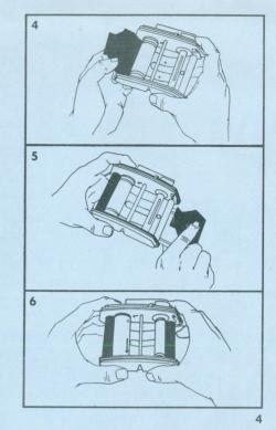
on the take-up spool is no longer felt. Film is now fully wound. Remove the full spool and transfer the empty spool to the take-up position. Carriage is ready for re-loading.
