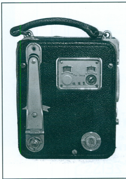
The intermediate variant with accessory shoe directly over the lens. This particular example has the distance scale in feet, a Sonnar f/2 1 cm lens, and serial number W52356. “Made in Germany” is engraved in English on the accessory shoe and in Chinese characters on the side. Figure 6
