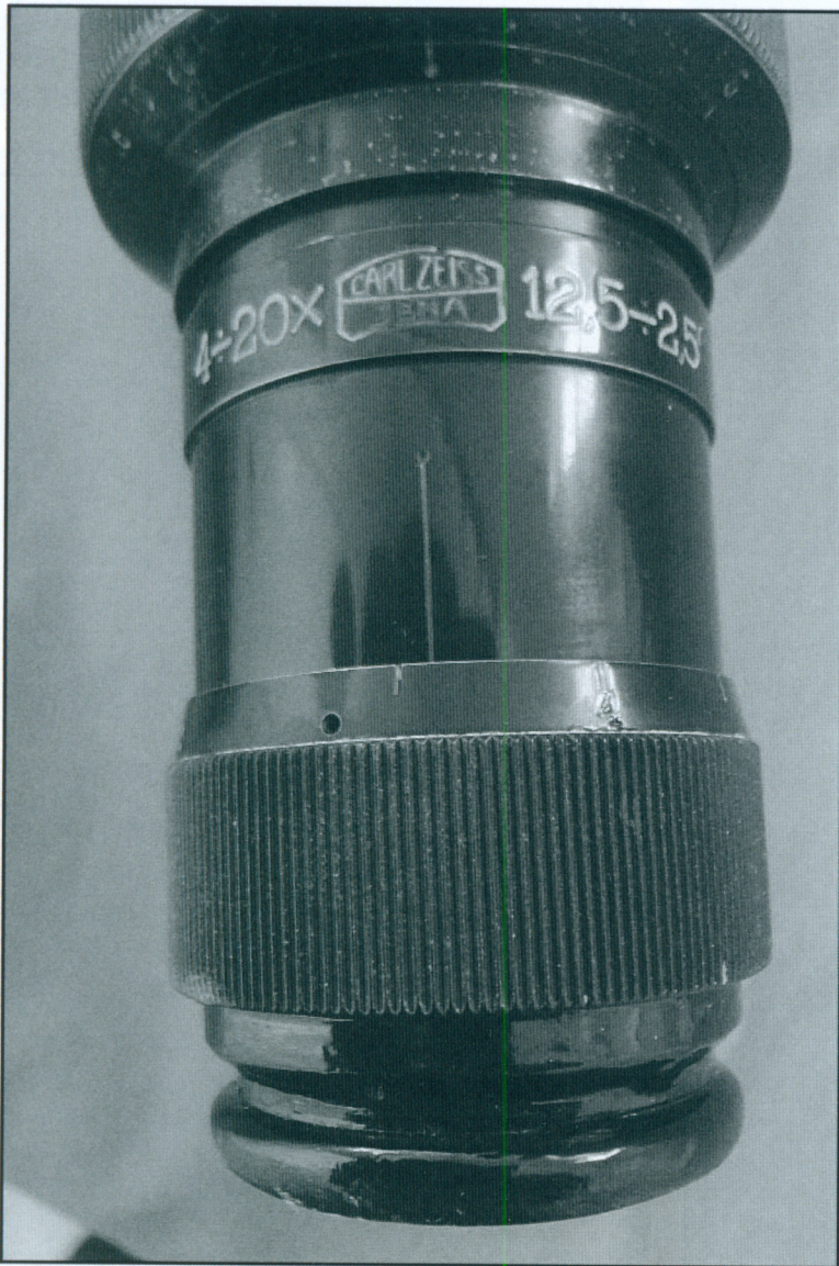
The eyepiece area , with focusing at the bottom, the 4× to 20× zoom range indicated, and the zoom control ring at the top. Figure 3
