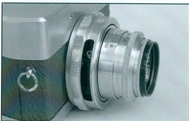
The prototype Werra , the smallest of all the models, seen here in front, back and side views. The lens, a 50 mm f/2.8 Novitar, is also a prototype, or "Versuch," experimental design. Note in the side view that the flash synchronization socket is on the lens ring and not on the camera body (near where the neckstrap attachment is here) as is the case with later models. Figure 1
