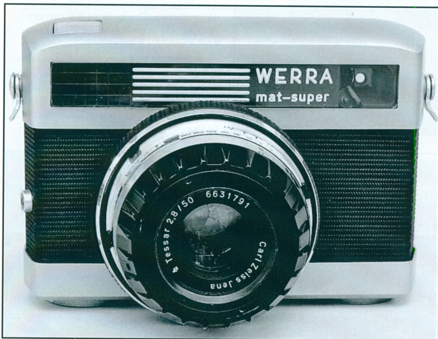
The Werra mat-super — the last of the Werra line. The back (shown below left) has, on the right, the shutter release sliding lever. The button marked “A” in the middle turns off the automatic exposure feature and allows manual settings using the rings visible on the picture, below right, around the lens.
