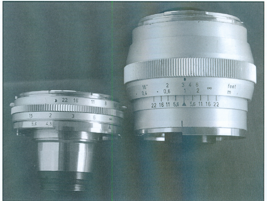
The f/4.5 21 mm Biogon (left) and the f/2.8 25 mm Distagon (right), both with Contax mounts. The Biogon is nearly as long overall as the Distagon, but most of it lies inside the camera where it might interfere with an SLR mirror. Figure 5
