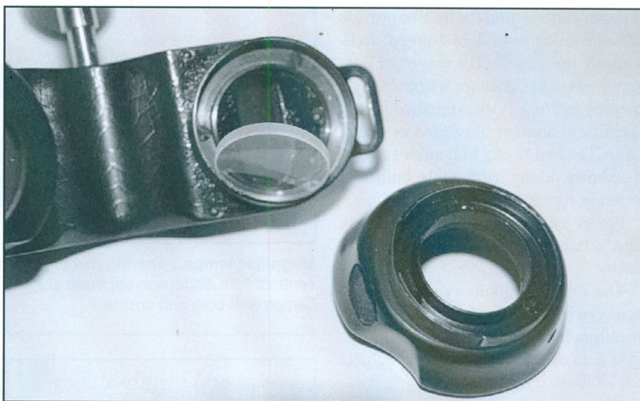
One of a pair of magnifier lenses of 2\times power (top center of the photograph), shown leaning out of its receptacle, with the eye cup and retaining ring at the side. Figure 1
