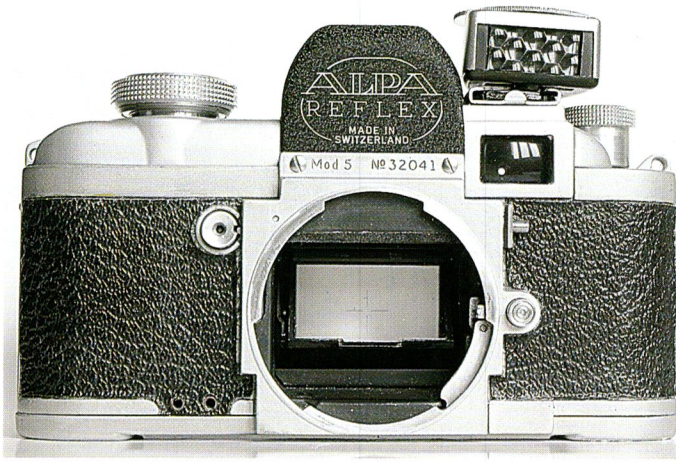
Alpha 5 without lens - from front - with new body, optical finder moved to the left, shutter release button on the front, pentaprism finder still has 45° eyepiece and a small exposure meter accessory is mounted on the shoe
