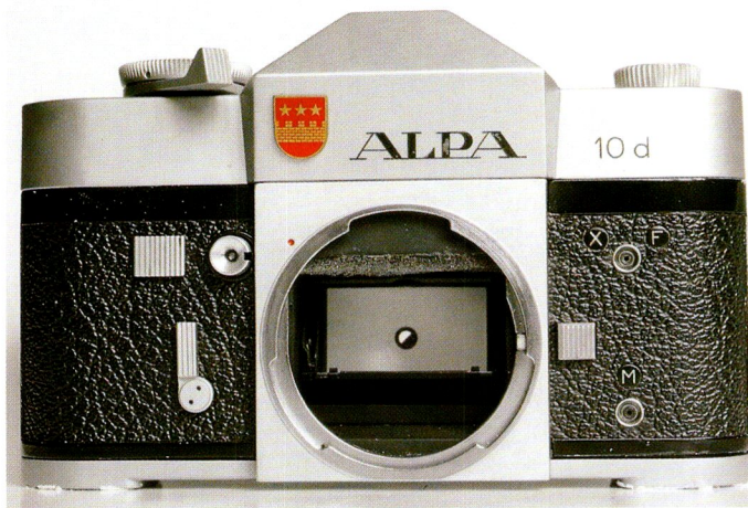
Alpa 10d with chrome finish without lens - from front - new linear design body and new controls except for lens catch and shutter release button on front that remained unchanged
