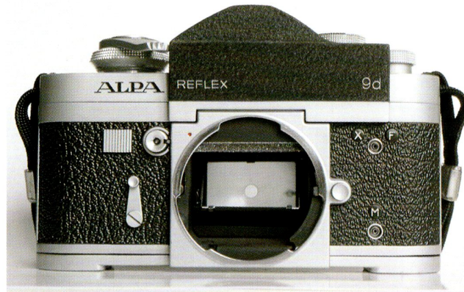
Alpa 9d without lens with chrome finish - from front - similar to Alpa 6c but with CdS TTL exposure meter
