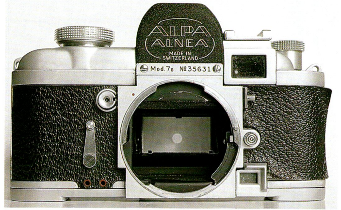
Alpha 7s without lens - from front - identical to the Alpha 7 complete with vertical base rangefinder and with exposure meter on the reflex finder focusing window; also marketed as the Alpha 8
