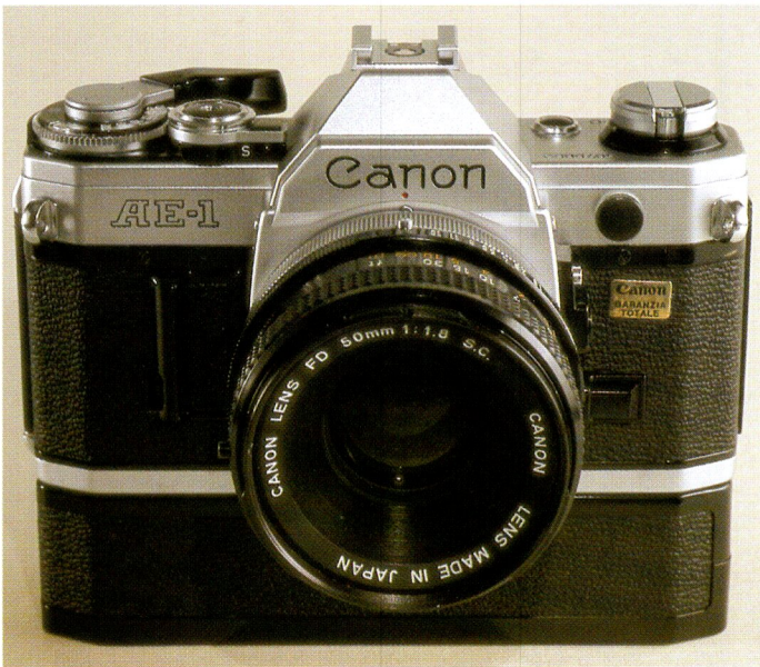
Canon AE1 with winder and standard 50mm f/1.8 lens
