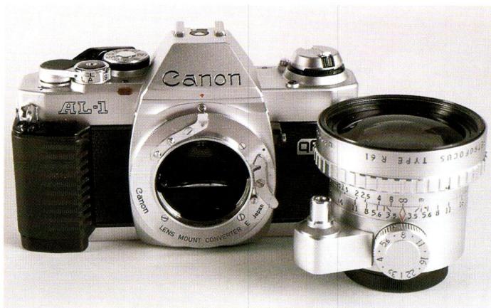
Canon AL1 with adapter ring and Angenieux Retrofocus lens for Exakta
