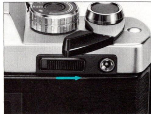
To prevent battery power drain, make it a rule to switch off the Check Button when in locked position by returning the film advance lever fully each time after exposure checking.
