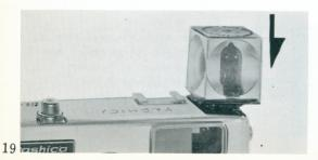
Press down the Flashcube until it snap-locks in place with one of its four sides facing towards in its detent position for firing.
