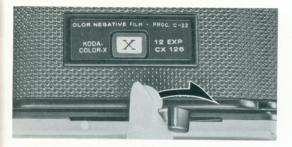
I After the last picture, operate Film Advance Lever until it locks. An "X" that appears in the window indicates that the film has been exposed. Don't remove the cartridge from the camera until all the yellow paper with "Xs" has been moved past the window; otherwise several exposures will be "light-fogged."
