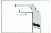
When you take pictures in the brilliant sunshine at the beach or in snow, you may find Exposure Pointer indicates the over-exposure. You can correct it by using a neutral density (ND) filter for color film and black & white film or Y2 (Yellow) filter for black & white film.
