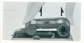
2 Slide down Lock Lever and open the back cover. Remove the cartridge and close the back cover.
