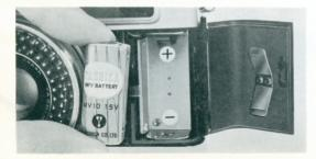
Drop in the battery (Mallory M504 or Eveready 504) plus(+) polarity up: minus (--) polarity *down* - as illustrated. Close the cover securely.
