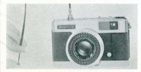
The "B" setting is used for taking pictures with a longer exposure than 1/30 sec. Rotate Lens Opening Ring until "B" is opposite the red line and the lens opening is automatically set at f/1.9. The use of a cable release and a tripod is recommended.
