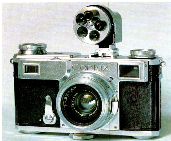
Biogon 3.5cm f/2.8 mounted on a Contax II equipped with the 436/7 multifocal viewfinder.
