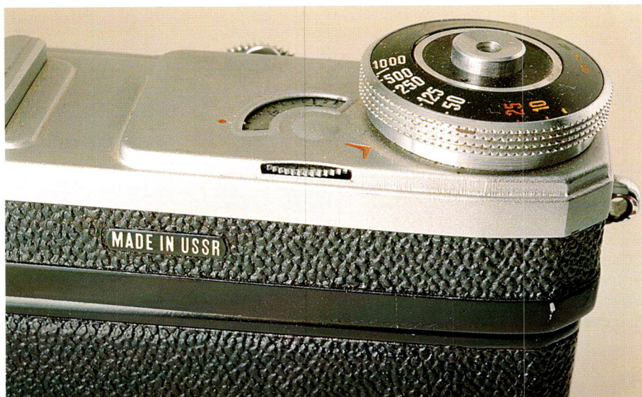
Kiev 4am: speed control, detail.
