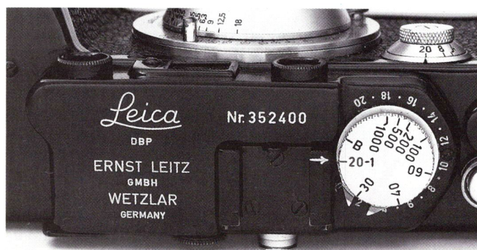
Reporter Nr. 352400 (1941) rebuilt in the 1950's. Note f-series flash synchronization and all capital letter engraving.
