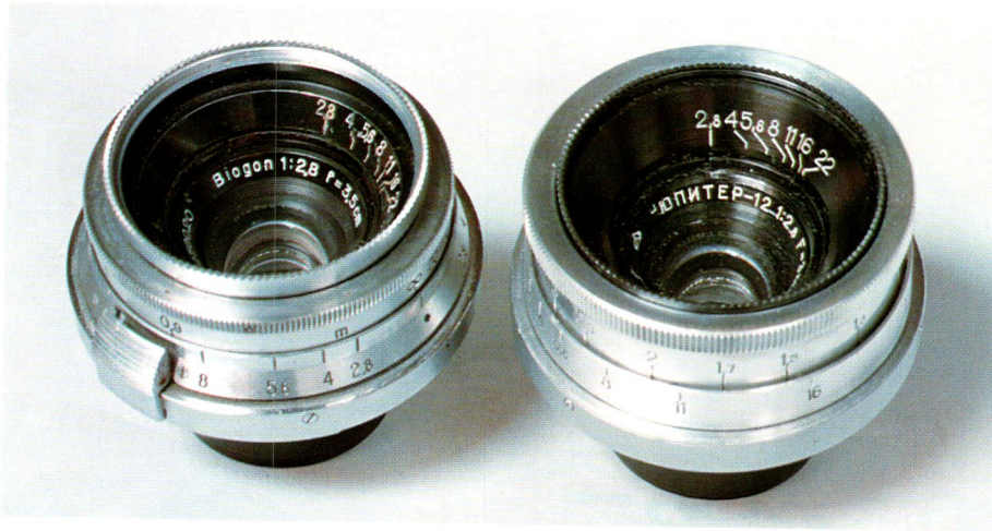
Left: Biogon 3.5cm f/2.8; Right: the Russian copy called Jupiter 12.
