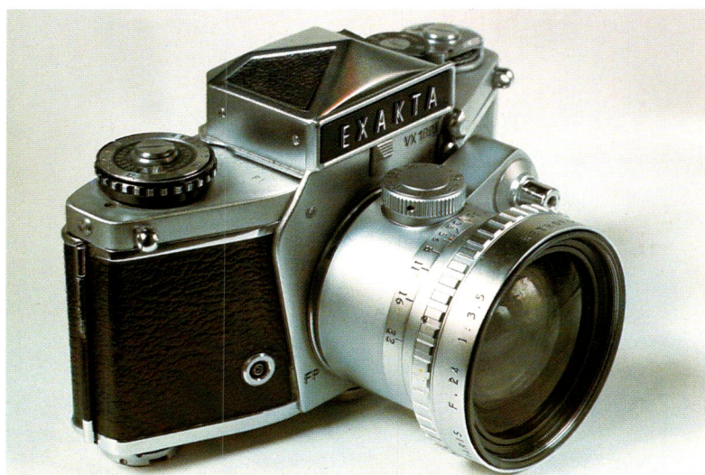
Automatic Retrofocus 24mm f/3.5 lens mounted on Exakta Varex 1000 with brushed finish, upper knob for aperture setting and aperture closure button connected to the camera shutter release button.
