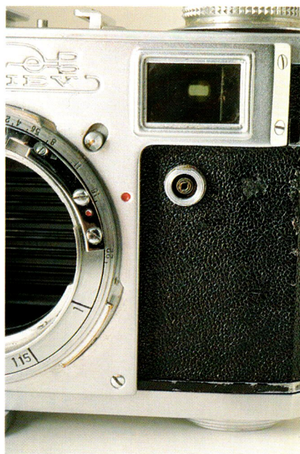
Kiev 2a: synch socket, detail.
