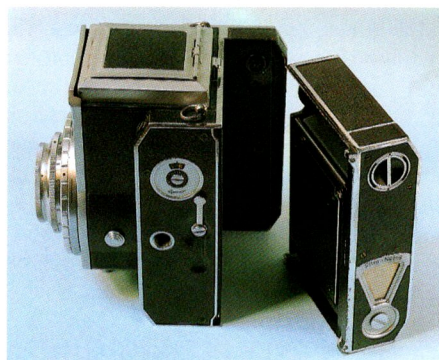
Film magazine removed; note the position of the release lever on the camera body.
