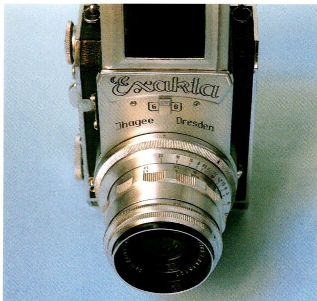
The camera minus the viewfinder and film back. Note the peculiar two-part mirror construction.
