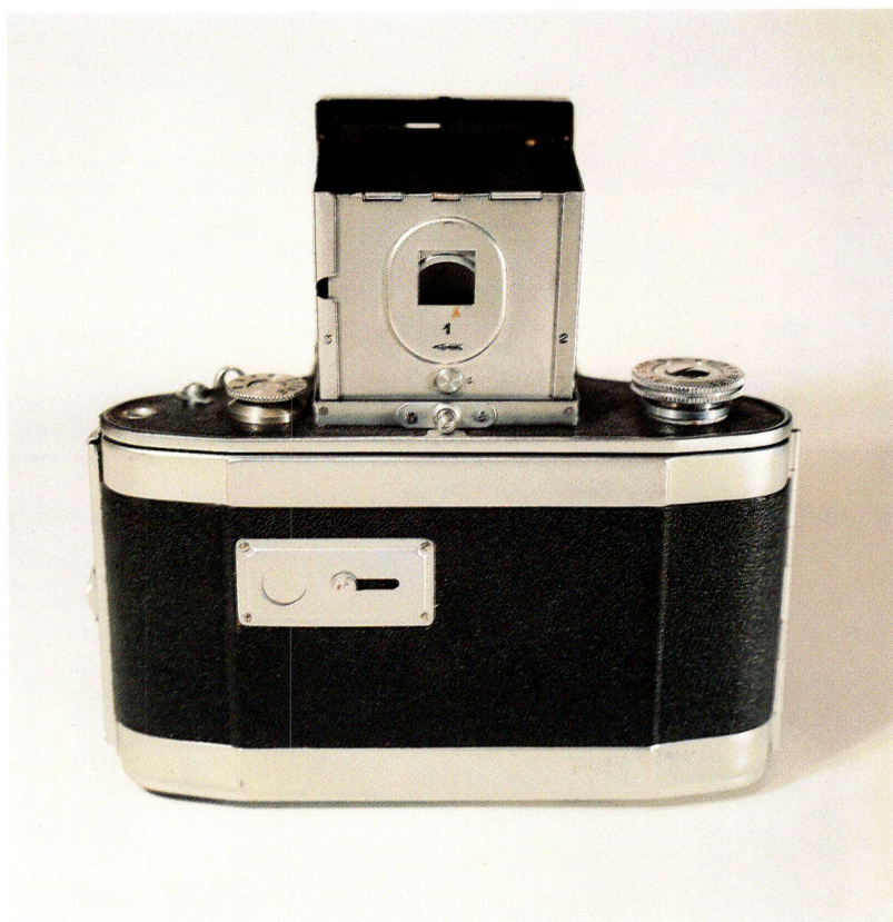
Rear view with closed back, note the small window to check film transport
