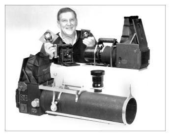
Jim is holding a standard Home Portrait lens in his right hand, and a standard 4x5 R.B. Series D lens in his left hand. To his left is a "Baby Bertha with a 16" f/4.5 Carl Zeiss Tessar, and in front is a Big Bertha with a 40" lens fitted on a Home Portrait. For scale, a  $3\frac{1}{4}$  x  $4\frac{1}{4}$  Speed Graphic is just in front of Jim.
