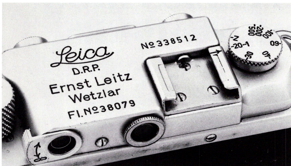
Leica III n. 338512 (1939) with Fl. n. 38079 engraving. Earlier cameras are usually marked Fl. n. 38078. The Fl. number is a Luftwaffe (air force) equipment inventory number.
