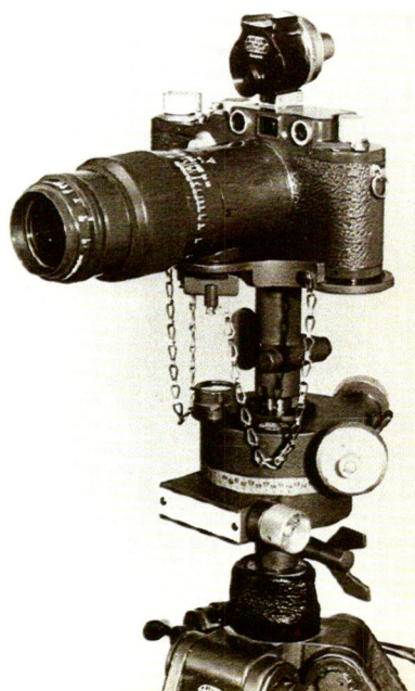
Ernst Leitz Wetzlar photo (1941) showing camera, 13.5cm 1:4.5 Hektor lens, reversed VIOOH viewfinder, support cradle, panoramic head and tripod. This unusual assembly is officially referred to as Kriegsgerate Rundbildkamera (military panoramic camera).
