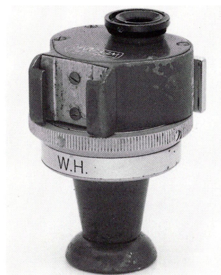
Grey W.H. (Wehrmacht-Heer) VIOOH viewfinder with eyecup. Designed to be used reversed in camera accessory shoe. Shows coverage for 13.5cm 1:4.5 Hektor lens.
