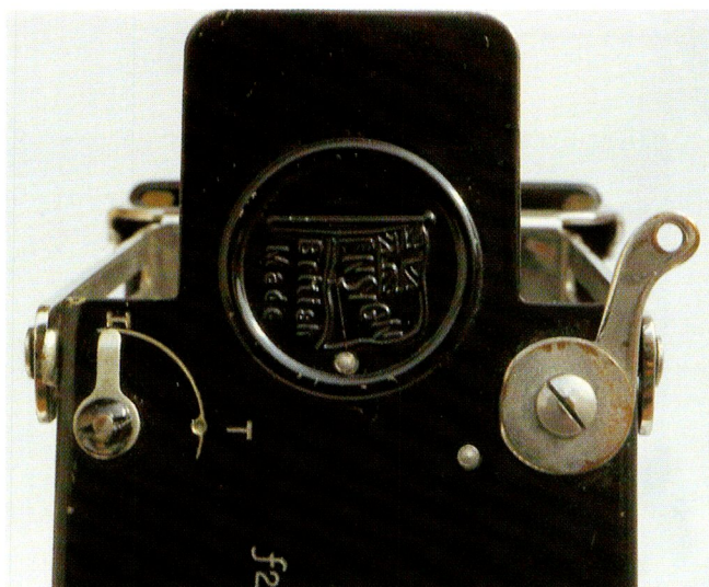
Ensignette no. 2: detail of front Ensign logo in relief, snapshot and T setting control and shutter release lever
