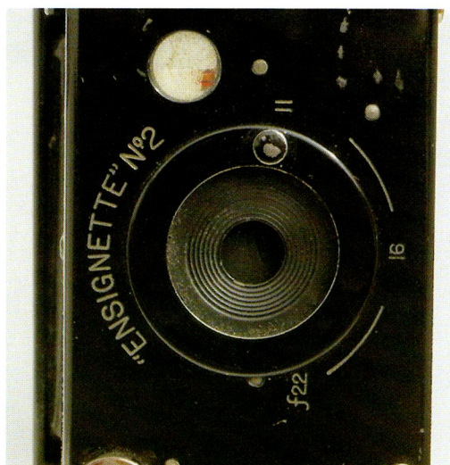
Ensignette no. 2: detail of front with aperture control on values 11, 16 and 22
