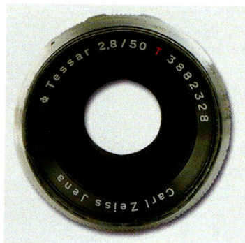
50mm f/2.8 Tessar no. 3882328 with diaphragm pre-set and aluminum finish (front view); note inscription "Tessar 2.8/50"
