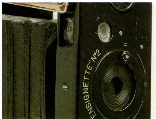
Ensignette no. 2: detail of front with viewfinder and lens opening
