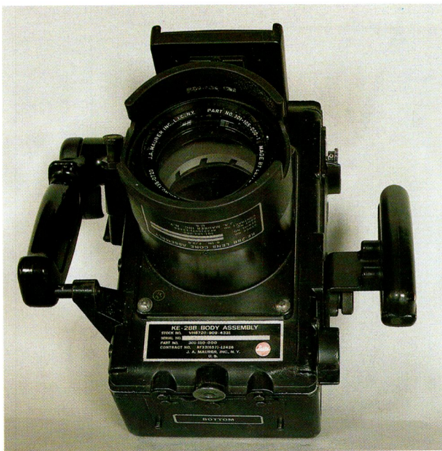
Camera seen from below with the unmistakable inscription "BOTTOM". Among the various markings on the ID plate is the unmistakable red Leitz logo, perhaps added later
