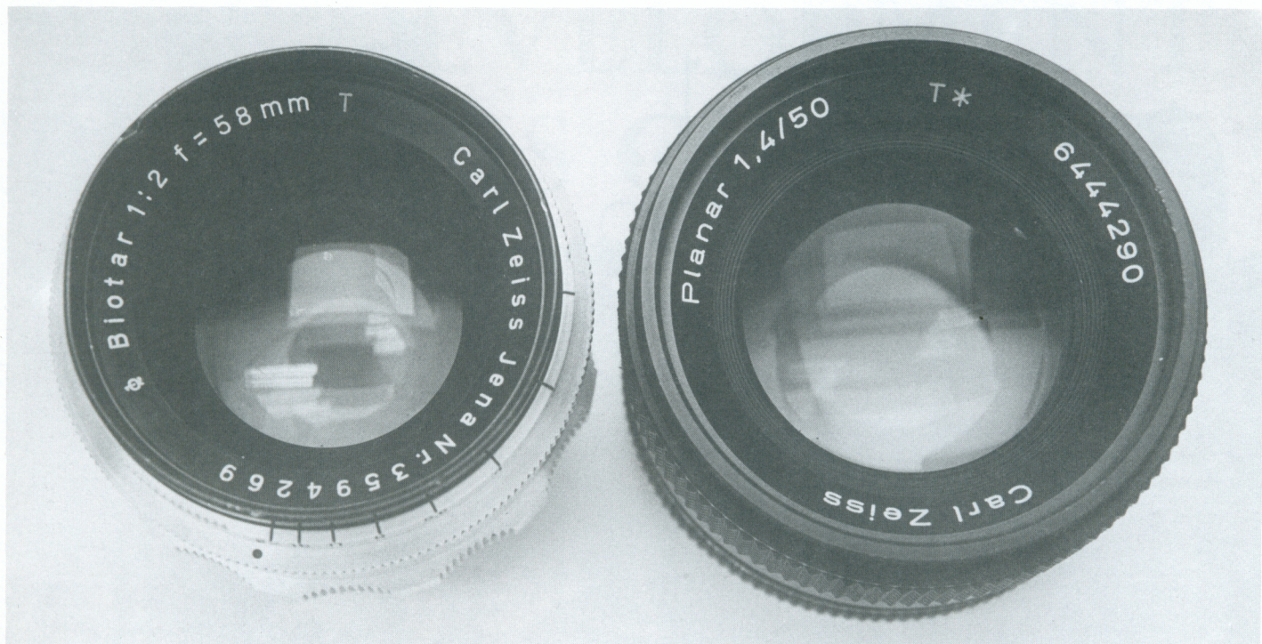
East German (Jena) T Coating from the early 'Fifties (left) compared with modern West German (Oberkochen) T* coating. Coating on the Biotar is single-layered, while T* coating is multi-layered.
