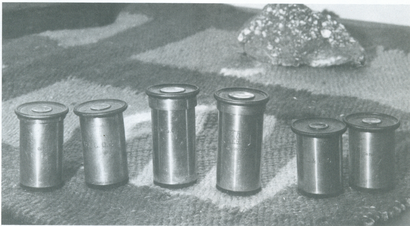
The three pairs of oculars carry both the Zeiss and B&L O.C. logos. Magnifications are not marked.
