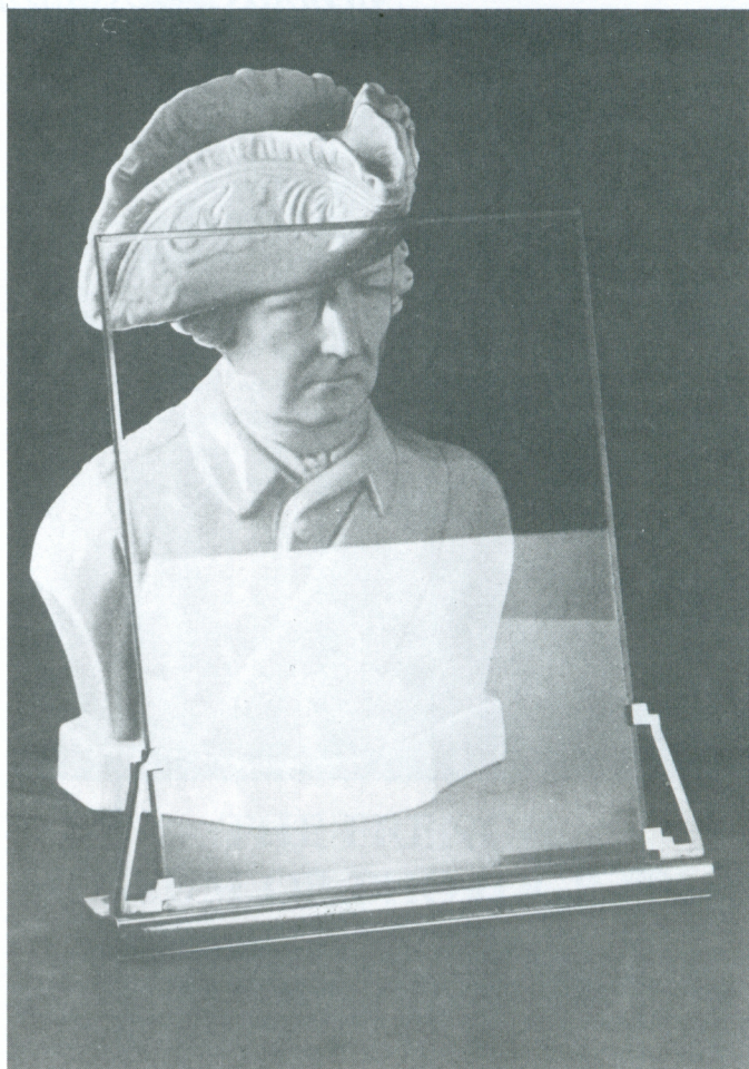
Upper half of glass is T-coated, lower portion is uncoated.
