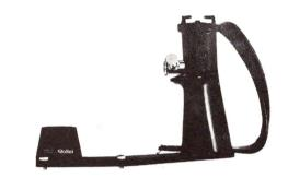
HAND GRIP WITH RELEASE—SL66. Left hand holds hand grip and operates focusing knob. Right hand works shutter time and crank. Has adjustable leather hand strap; removeable cable release allows releasing teleshots with left hand; has tripod coupling and dovetail camera (tripod) adapter; accepts flash bracket on bar; has accessory shoe on grip top. Cat. No. 208 930 (12432)
