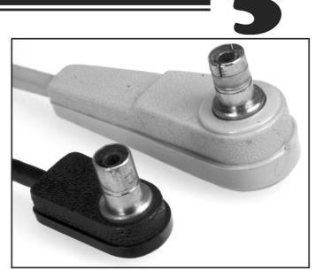
Fig. 6...Above...The cable plugs: at the front the 2-core version, and in the rear is the 3-core version.
