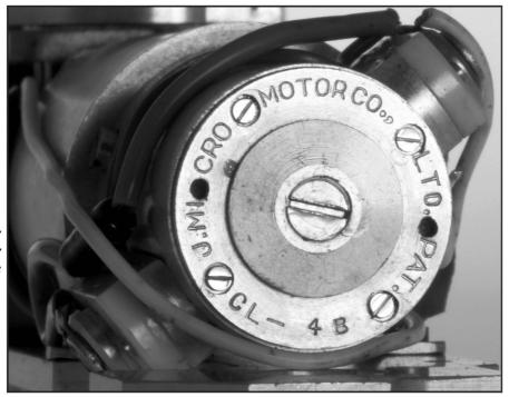
Fig. 8...right... The small electric motor used by Nikon in their famous motor drives. It is Micromotor type CL-4B.
