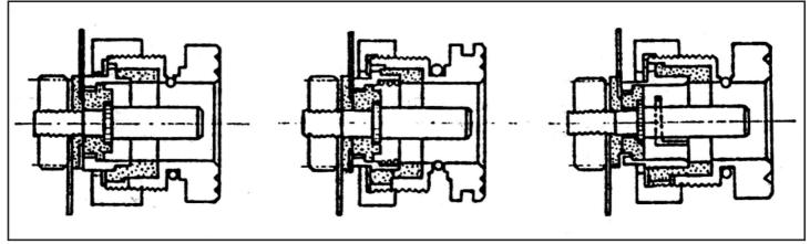
Fig. 7...Above... The improvement of the 3-core sockets. From left to right: the 1st version with 2 concentric triangular grooves on the face of the chrome ring; the 2nd version with an additional rectangular groove on the circumference (does not appear on battery packs); the 3rd version with only one triangular groove on the face, but now larger. (The chrome ring is on the right in each type)
