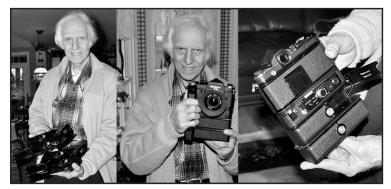
*Pic 1...left...Matching MD-100A motor drive and MF-1A 250 shot bulk back , but the wrong MB-100A battery pack.*
