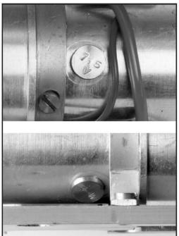
Figs. 9 & 10 Fig. 9...Left...Details of Micromotor type CL-4B, stamped 7.5V, 2W.
