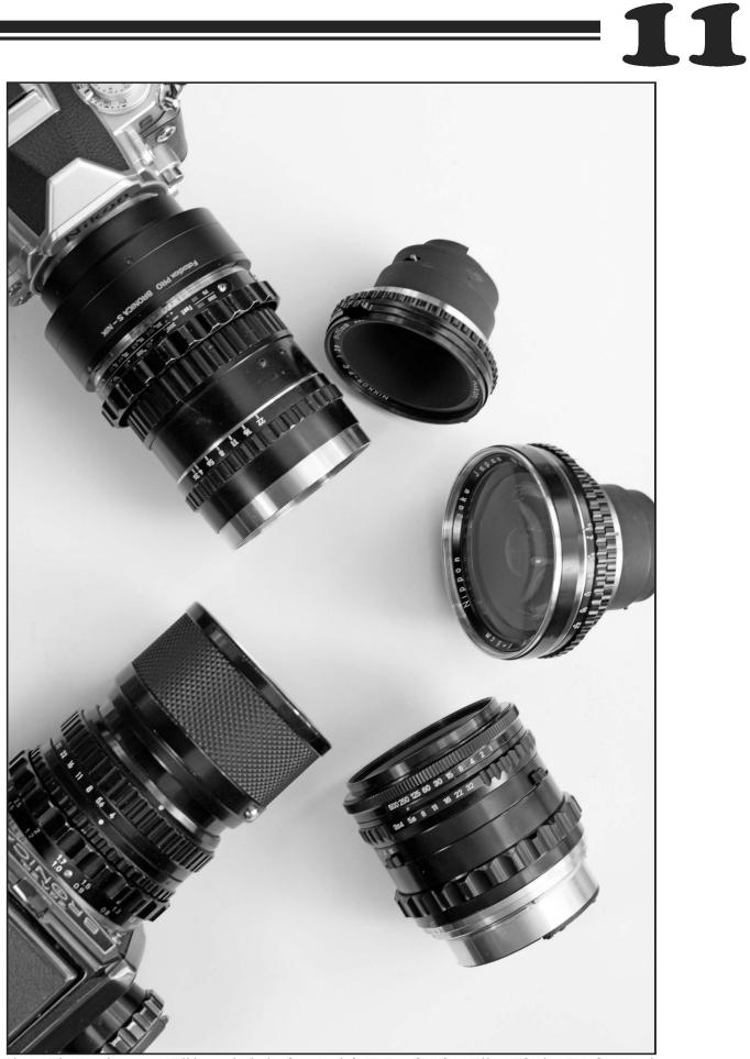
Fig. 1...The Bronica-mount Nikkors, clockwise from top left: 13.5cm/f3.5 Q on Nikon Df using Fotofiox Bronica S to Nikon adapter; 75mm/f2.8 PC; 5cm/f3.5 H; 105mm/f3.5 Q Synchro; and 200mm/f4 P on a Bronica S2A.
