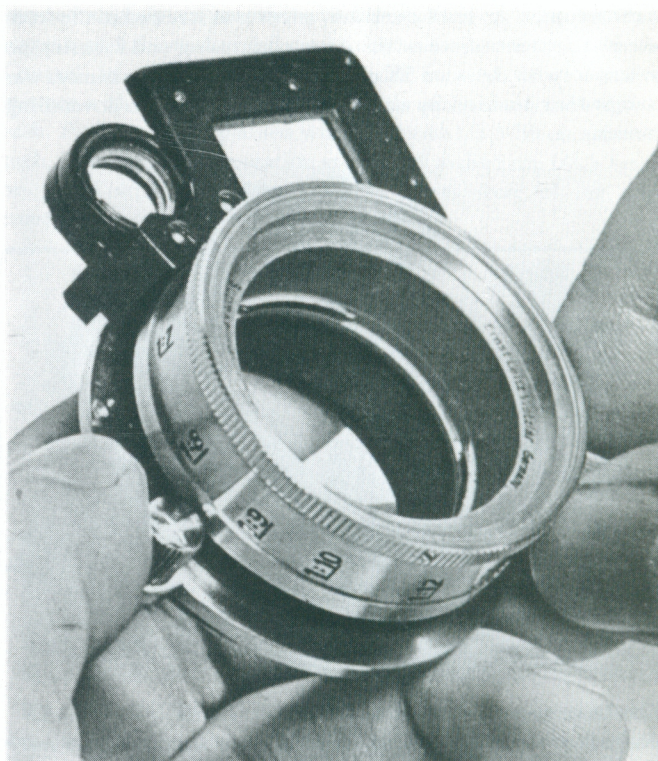
The Optical Short Distance Focusing Device (NOOKY), interposed between the Leica and a 5 cm. collapsible lens, permitted rangefinder focusing and parallax corrected viewing from 3.5 feet to 16.5 inches. A scale on the mount enabled photographs to be taken with predetermined image: object ratios.
