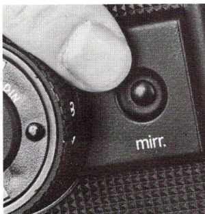
Mirror may be pre-released with this button (or locked up with ME-1 for multi-exposures) but lens apertures must be set manually as camera photo cells are blocked when mirror's in up position.
