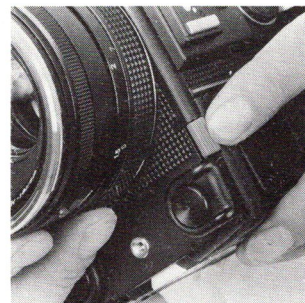
Red color-coded lens release permits easy 45° counterclockwise lens release. Note finger guiding rim on "1", hand shutter release, socket for cable release.
