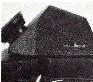
Press this latch (and its mate on other side) and finders slide forward for removal without removing back. 45° prism, fixed hood with magnifier, and standard folding hoods are available alternatives.
