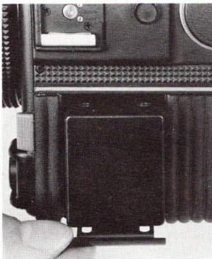
Quick-rechargeable 9.6-v nicad powers 6006 for 600-800 film exposure/advance cycles at normal temperatures.
