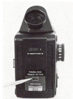
Move darkslide tab to bottom, opening magazine and switching on camera. S in counter window shows back is loaded. Tap either release once or twice and film winds on and counter below film-box-end clip stops at "1."
