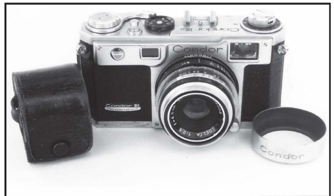
Bottom 2 photos...This is the later, more upscale, Condor III S, with a rewind assembly even more S2-like. However, the top plate step is less like the S2 but the front plate is still a match for the Nikon's.
