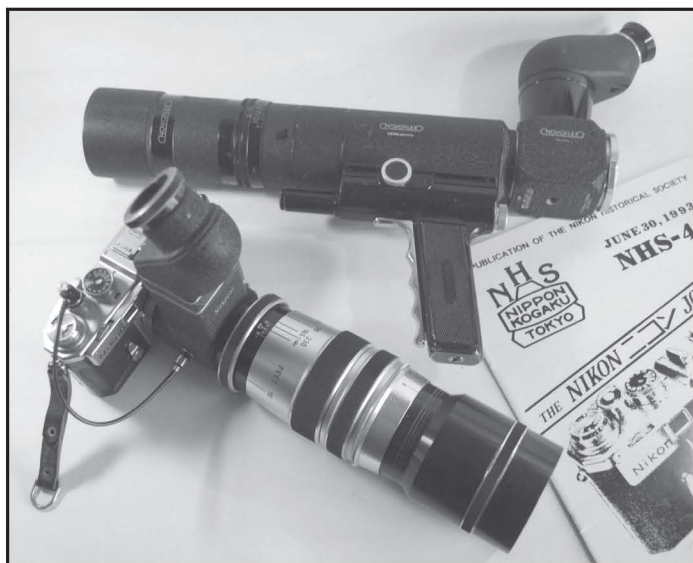
The Kilfitt Kilfascope mounted on an SP with the 300mm/f5.6 Kilar in front. Behind is the Novoflex housing in Contax mount with the 300mm/f5.6 Noflexar lens
