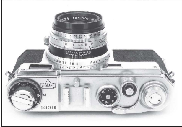
Above 2 photos...Views of the standard Condor model, which came with a 4.5cm/f2.8 Condor Delta lens. Note that the interior resembles the Nikon S2's four film guide rails. Also, more visible in these shots, the top controls and the front decorator plate.
