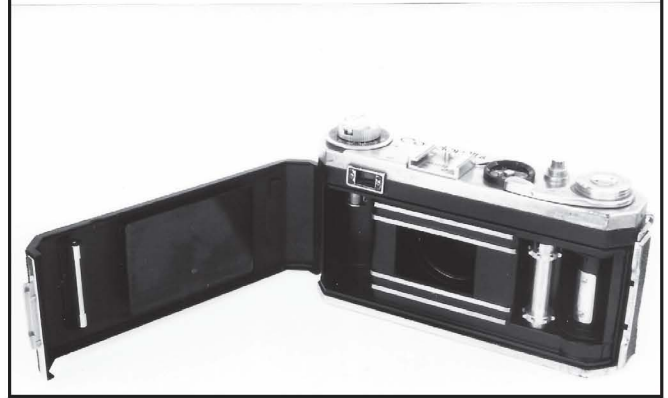
Bottom 2 photos...This is the later, more upscale, Condor III S, with a rewind assembly even more S2-like. However, the top plate step is less like the S2 but the front plate is still a match for the Nikon's.
