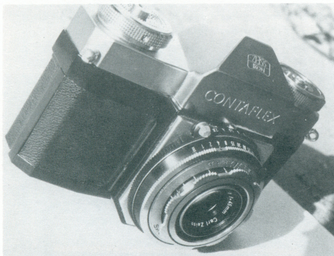
Early Contaflex I with type C f-stop lever.
