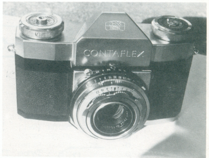
Later Contaflex I body, serial L16871 with lens 1548075. The body is casting type III with f-stop type D.
