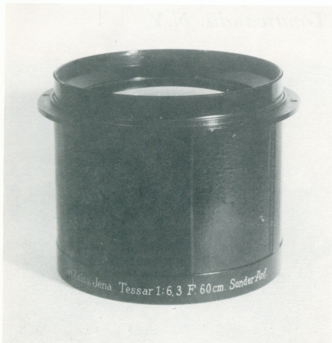
Custom-made 60 cm. f6.3 Tessar, engraved "Sonder-Anf." Abbreviation stands for "Sonderanfertigung" or "Special Production."
