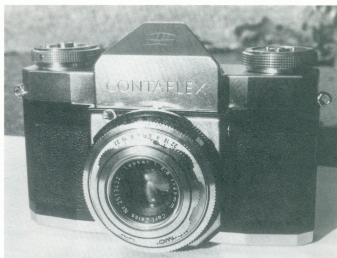
Latest Contaflex I with type D f-stop lever. This example is body serial R41668 and lens 2513422.
