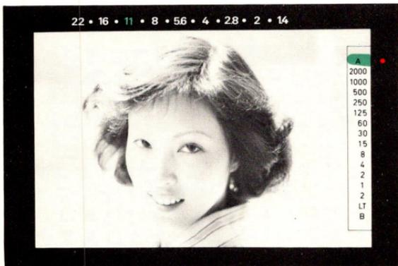
2. When the LED dot comes on in alignment with 'A', stop down the lens aperture so that the LED dot aligns with 2000 (1/2000 sec.) or smaller figure.
