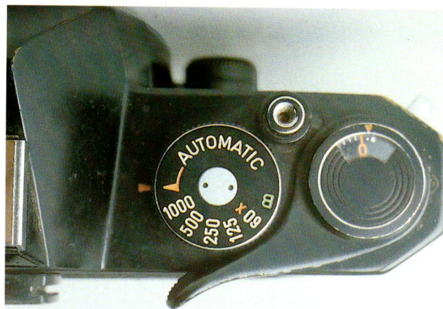
Asahi Pentax ES: a detail of the shutter speed selector.
