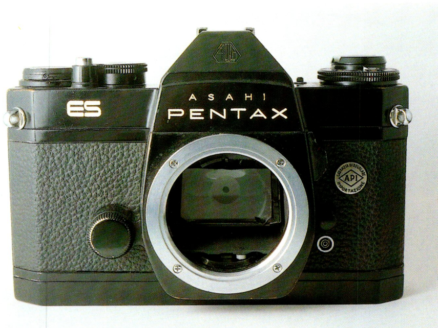
Asahi Pentax ES minus lens, with screw mount in evidence.
