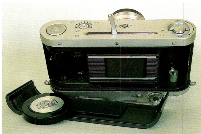
Henso Reporter with open back and German language indications (AUF and ZU) on the camera back release.
