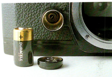
Asahi Pentax ES: a detail of the 6V battery.
