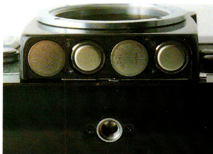
Asahi Pentax ES II: a detail of the four 1.5V batteries.
