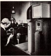
The DSA/Senrac dries roll film right on your stainless steel processing reels in 2 minutes. Filtered, temperature controlled air sweeps film dry without dust or drying marks.
