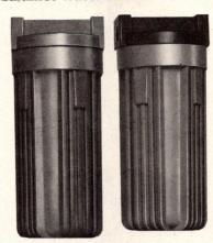
Water filter housings made from tough polypropylene with talc filled walls for greater insulation. The cold water filter housing is rated at 125 psi at 125°F; the hot water filter housing is rated at 200 psi at 200°F. Either filter housing can be installed easily on new or existing plumbing. 34″ NPT inlet and outlet.
