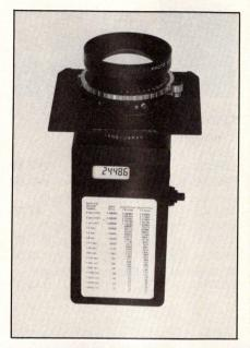
bulb or bright area), place the probe near the center of the film plane or near the rear element on a leaf shutter lens, and release the cocked shutter. The Shutter Tester will display the shutter speed in seconds (i.e., 0.00100 is 1/1000 of a second) and will automatically reset. It's very easy, it's very accurate, and it's very inexpensive.
