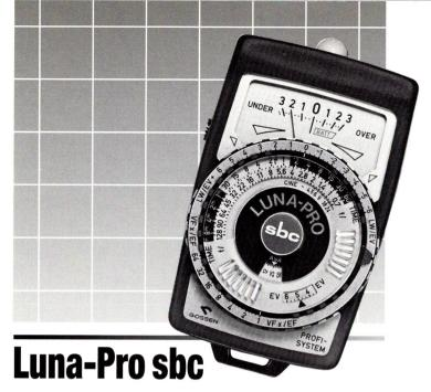
Featuring the latest generation silicon blue cell, the Luna Pro sbc reads accurately down to -4 EV for extreme low light capability. It features the accurate Null metering system, take one reading, center the indicating needle pointer with the outer ring of the scale and see not only an exposure reading, but all of the other lens and shutter settings possible at that light level.
