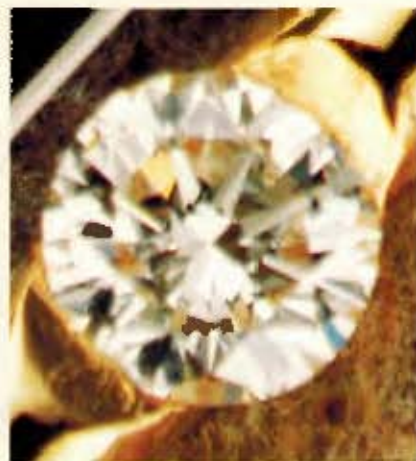
Fig. 10 Detail, magnification 10 times with SINARON-S 360 mm, results in lower edge definition than fig. 9
