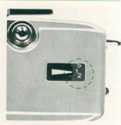
The film counter shows S, 1, 2, 4 and subsequent even numbers up to 36. The numbers 12, 20 and 36 are in yellow color. Each time the film is advanced, the counter counts up the number of exposures made, which is pointed by the orange color arrow (). When the rear cover is opened, the counter returns automatically to S.
