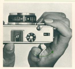
Advance film and release shutter until No. 1 appears in exposure counter window.
