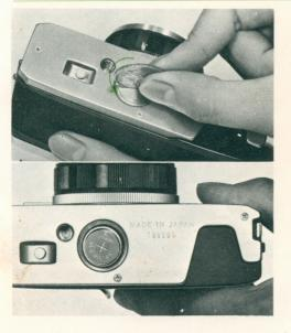
For correct camera operation, the mercury battery must be properly inserted into the battery compartment at the bottom of the camera.
