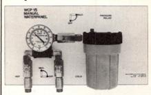
The WCP 15 panel provides economical temperature control. It features separate hot and cold water adjustment valves for temperature mixing, preplumbed 3" dial thermometer, flow control valve, ½" N.P.T. inlet connections, ¾" garden hose outlet connection, and a 30 micron reuseable water filter. The unit is supplied on a convenient to mount wall panel. Accessories include optional vacuum breaker and spray hose which require user installation.
