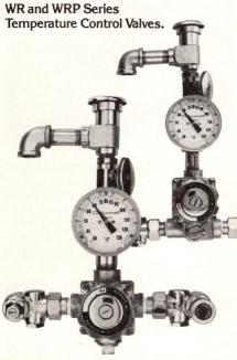
Eliminate time consuming adjustments in mixing hot and cold water for proper temperature. Calumet's temperature controls mix and regulate output temperature and hold it to ½° of the desired setting. They feature an accurate dial thermometer and a thermostatic motor. Each temperature control includes thermostatic valve, plumbing fittings, flow control valve, shut-off valve, check stops with strainers and indicating thermometer with recalibration screw setting.
