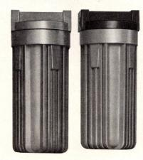
Water filter housings made from tough polypropylene with talc filled walls for greater insulation. The cold water filter housing is rated at 125 psi at 125°F; the hot water filter housing is rated at 200 psi at 200°F. Either filter housing can be installed easily on new or existing plumbing, 34" NPT inlet and outlet.
