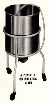
Deep drawn 10-gallon Type 304 photographic stainless steel tank has a powerful non-corrosive pump for recirculating and mixing photographic chemicals. Includes 6' of flexible plastic delivery hose coiled inside tank. Pump circulates at over 6 gallons per minute and is completely sealed against moisture and chemicals. Storage stand is equipped with casters for easy transfer of chemical from room to room. CP5011 . . . . . . . . \$299.95
