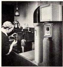
The DSA/Senrac dries roll film right on your stainless steel processing reels in as little as 2 minutes. Filtered, temperature controlled air sweeps film dry without dust or drying marks. Features built-in 10 min. timer with bell, warm or cool switch with internal thermostat, corrosion resistant construction with washable filter, weight 18 lbs., height 24," 115 volts, 615 watts with 8' power cord, capacity 3-120mm or 5-35mm reels or combination up to 8½." Includes wall mount.
