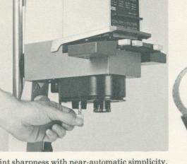
"Rangefinder" focus feature Assures critical print sharpness with near-automatic simplicity. Projects built-in target image onto baseboard. Image is red and green when out of focus, and turns white when focused sharply. Eliminates eyestrain and need for magnifier. Target swings out of the light path when not in use.
