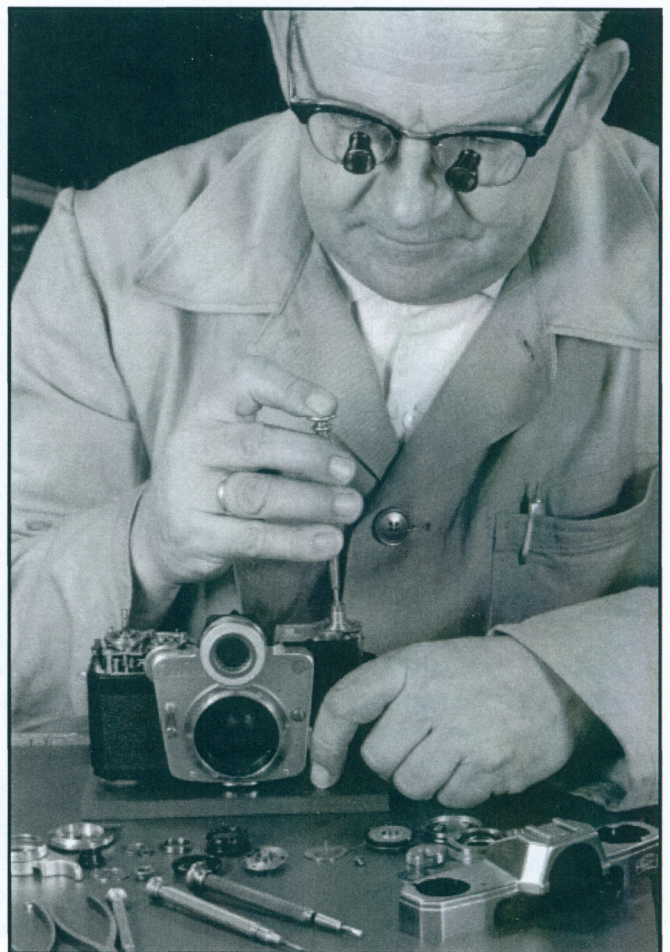
Assembling a Bullseye Contarex. The skilled hand work required to put together the 1,100 individual parts contributed to the high price of the camera. Figure 3
