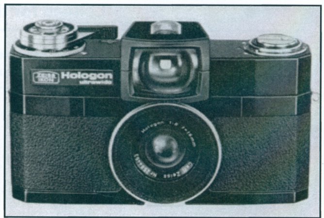
The Hologon Ultrawide , made for the 15mm f/8 Hologon lens with only 4.5mm clearance between lens and film. Figure 9
