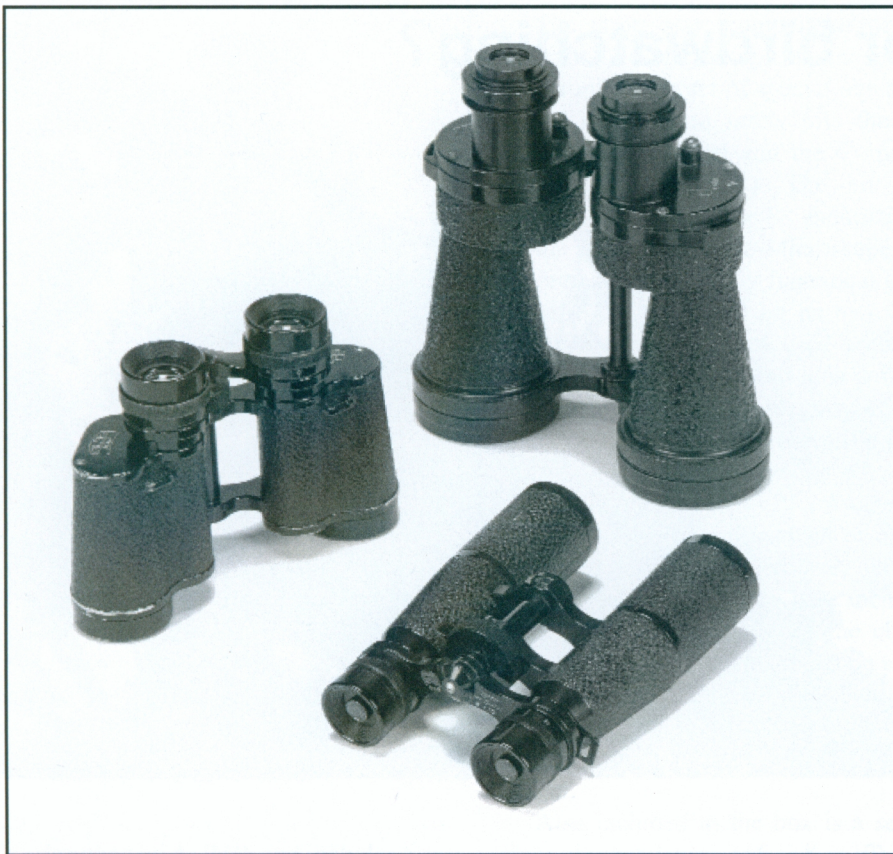
The three basic types of prismatic binoculars. Left and front, two binoculars with the same specifications, 8×30, but different prism systems. The one on the left is a Porro-I Carl Zeiss Jena Deltrinem 8×30 with uncoated lenses, serial number 1330466. In the foreground is a “Dachprisma” (roof-prism) Hensoldt Wetzlar D.R.P. Sport-Dialyt 8×30, uncoated lenses, serial number 251068. At the right rear is a Porro-II Ross London Mk. IV, 5×40, with coated lenses but without the large rubber eyeshield; serial number 6682. (All from the author’s collection.) Figure 2
