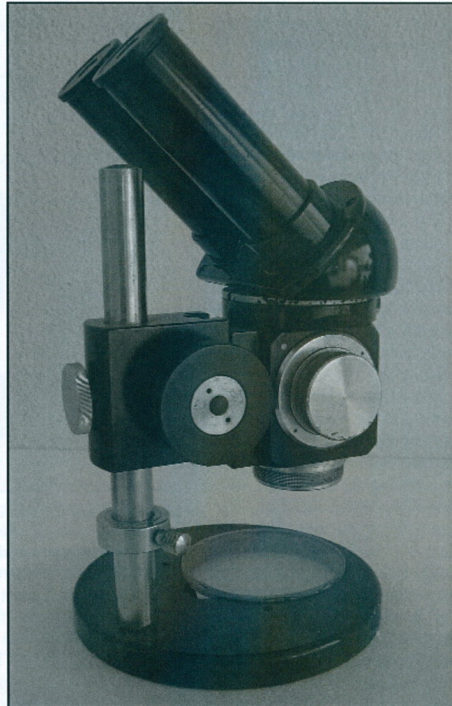
The Zeiss Opton Stereo Microscope , which became the Carl Zeiss Stereo Microscope after the "Opton" name was dropped in 1953. Figure 2
