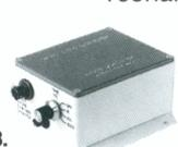
**1. Photo-Sonics IRIG Timing Pulse Generator, Model CTPG/LED.** Provides output from IRIB B or 10, 100 or 1000 pps coded internal clock plus circuit for event marks. Made especially to drive LED's, 115 VAC, 28 VDC power inputs or 12 VDC internal NiCad battery with built-in recharger.
