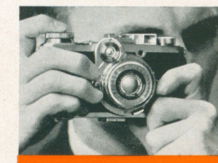
The Nettax range-finder is manipulated by rotating a lever. Like the Super Nettel, this camera can be focused on all objects from 3½ feet to infinity.
