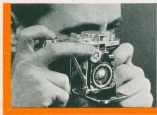
Moving a milled wheel with one finger adjusts range-finder and focuses the lens at same time... All controls are grouped on top of camera.
