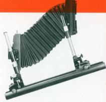
Tilting the monorail in combination with center tilts considerably increases the amount of vertical adjustments (rise and fall of camera back or lens standard).
