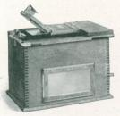
A N AUTOMATIC masking device on the top of the printer holds the negative firmly and gives the print a white margin. The light inside the box is switched on as the hinged top presses the paper in contact with the negative. A
