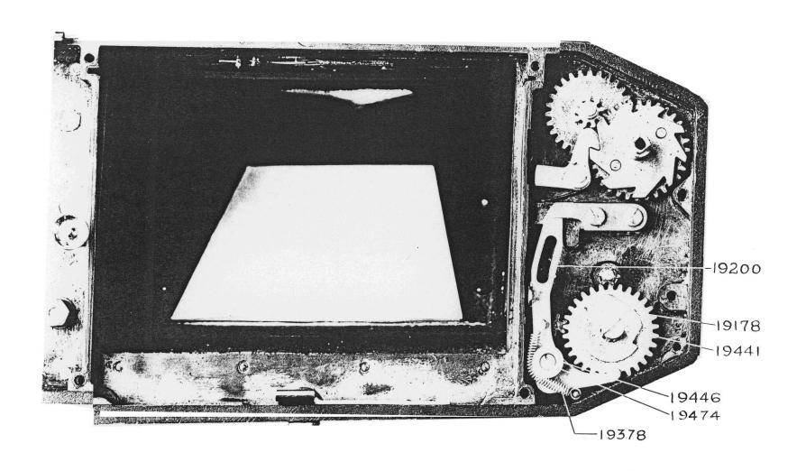
In the order given, remove spring #19431, spring #19432, stud #19320, locking catch #19383, and shutter setting catch #19201. The mechanism now appears as in:
