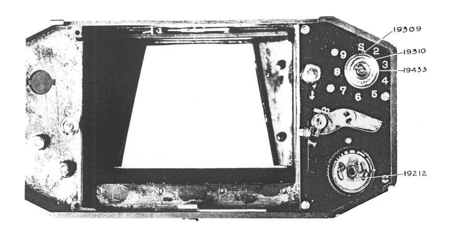
Illustration No. 6 reveals the shutter curtain slot adjustment plate assembly #19212. This also lifts out without further manipulation.
