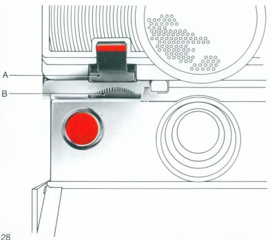
**To use the focus wheel:** Look at the most important part of the scene. Roll the wheel all the way in one direction, then all the way in the other. Notice that the image changes from fuzzy to sharp and back to fuzzy.
